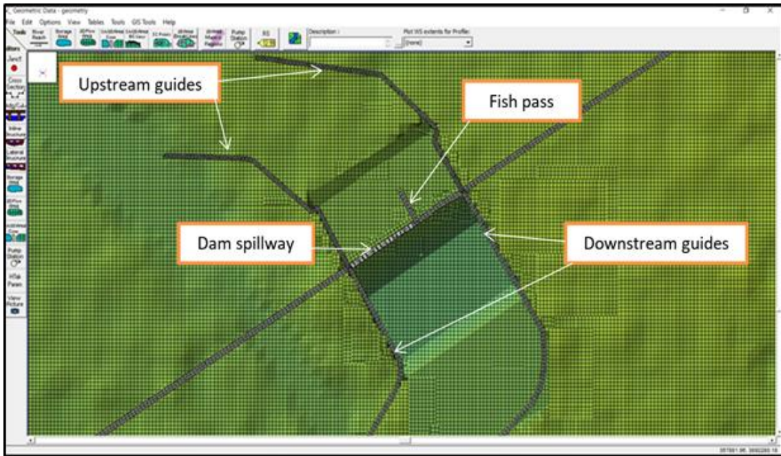
Figure (6): The representation of the Dam and Head Race Channel by the geometry window in the HEC -RAS Software as designed.
