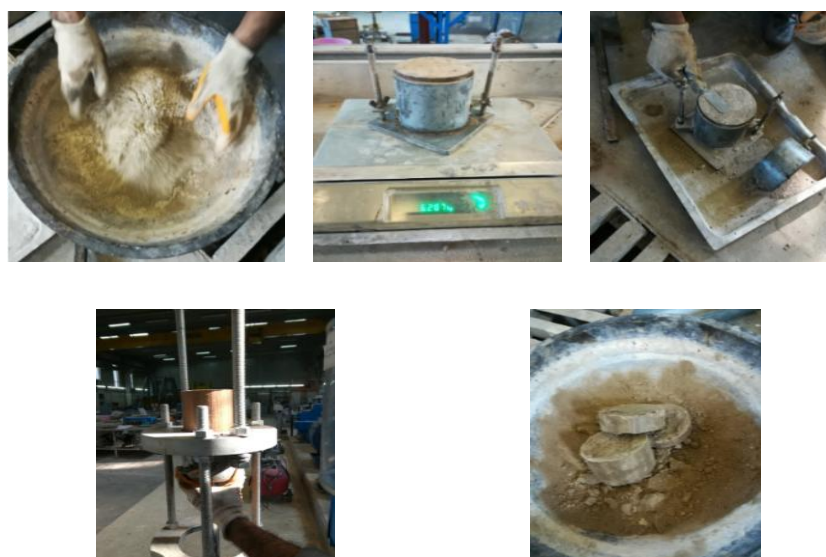
Figure (2): Compaction test for stabilized subgrade soil
