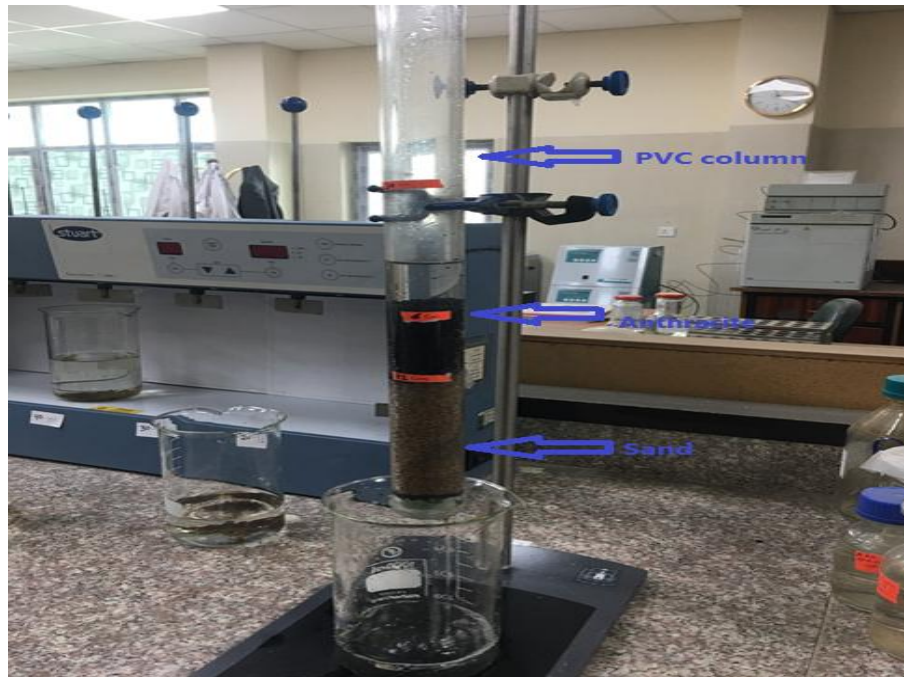
Figure (4): Laboratory sand filter designed by research team
