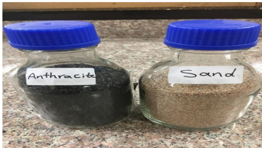
Figure (3): Media of sand filter
