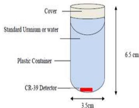
Figure (3): Special uranium dosimeters, to measure the uranium concentrations in the standard solution or water.
