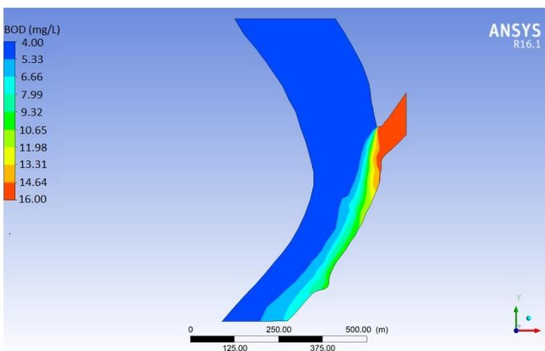
Figure (9) : Average flow,  $Q_{Diyala} = 62 \text{ m}^3/\text{s}$ ,  $Q_{Tigris} = 520 \text{ m}^3/\text{s}$ .
