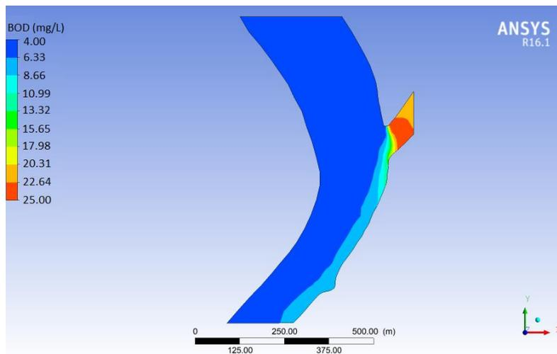
Figure (8) : Low flow,  $Q_{Diyala} = 5 \text{ m}^3/\text{s}$ ,  $Q_{Tigris} = 355 \text{ m}^3/\text{s}$ .
