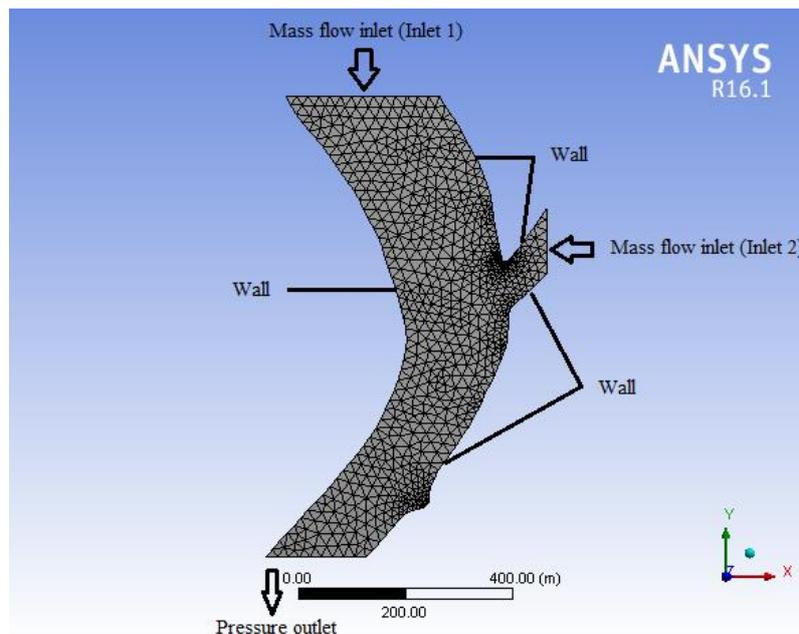
Figure (1) : Geometry, boundary condition and mesh of the study area.
