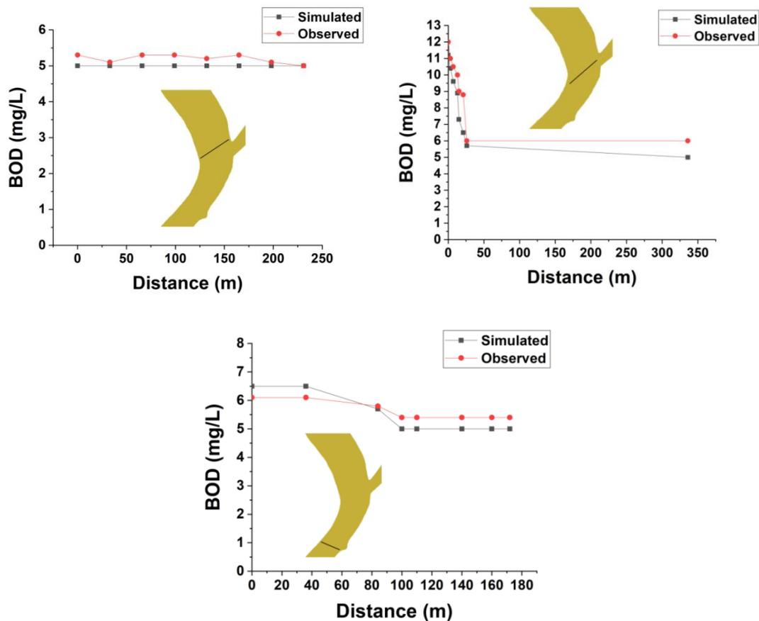
Figure (4) : Calibrated vs. Simulated results of BOD dispersion.
