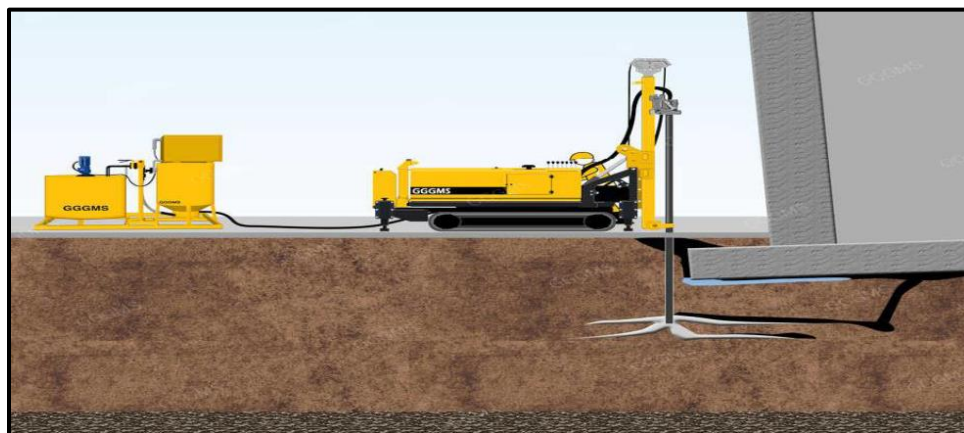
Figure (7): Fracture grouting (Chaitanya et al., 2023).
