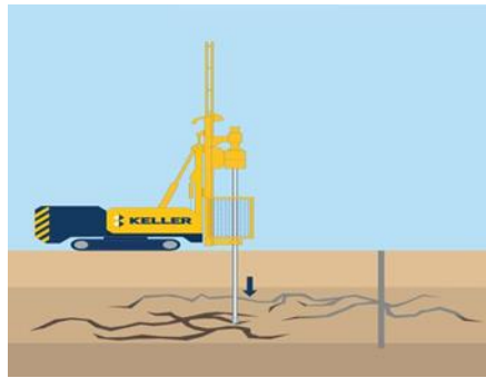
Figure (7): Rock grouting
